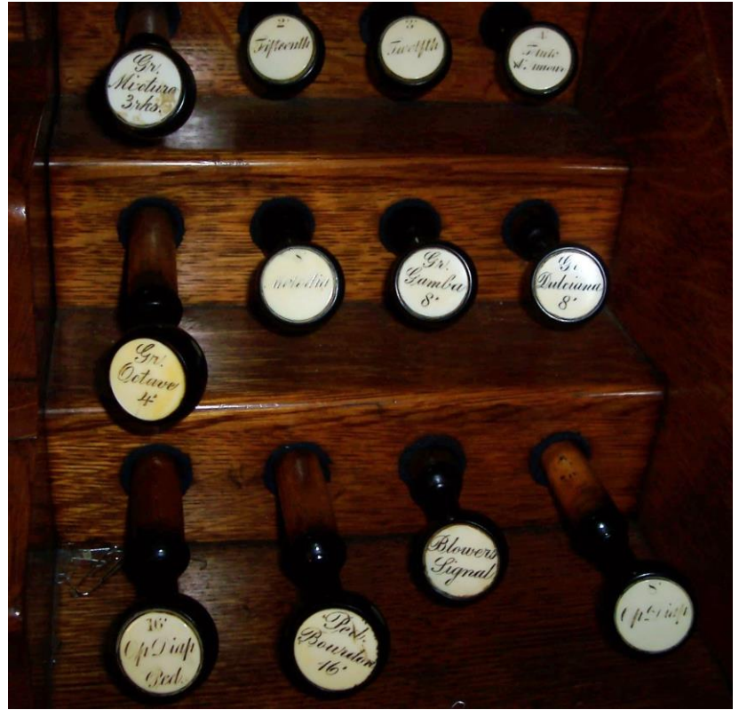
The Great and Pedal stop knobs with the Blowers Signal. The stop names on the faces (showing the pitch-length first) are thicker and more faded than the other (original) faces.
