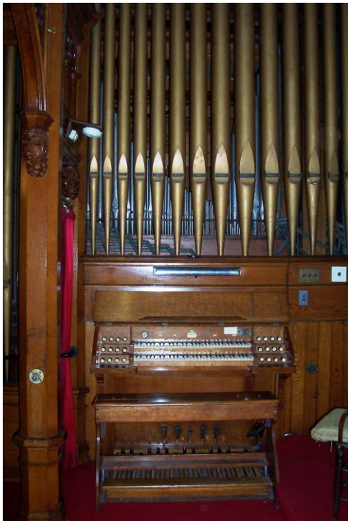
A front view showing the keydesk, stops, bench, pedals and façade pipes. Behind the façade you can see the silvery interior pipework.
