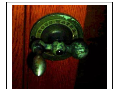
A handle for the water motor that at one time operated the bellows.
