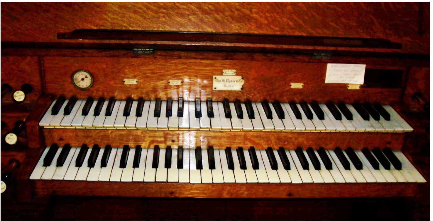
The small rectangular plaques above the Swell manual correspond to the composition pedals (metal foot levers) above the pedalboard (below). They read, in order from l.-r.: Swell Piano , Swell Forte , Gt. to Ped. , Great Piano , Great Forte
